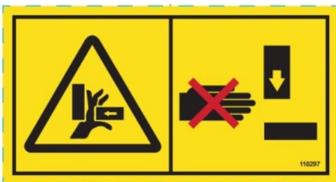
Decal #110297 Be careful of pinch points, do not put hands or any other part of the body into moving parts.
