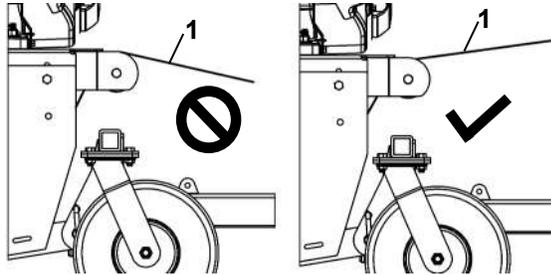
6. In the case the winch is not strong enough to lift the snowblower or if the top of the pulley is higher than the winch, it is possible to install the lift system as follows:
